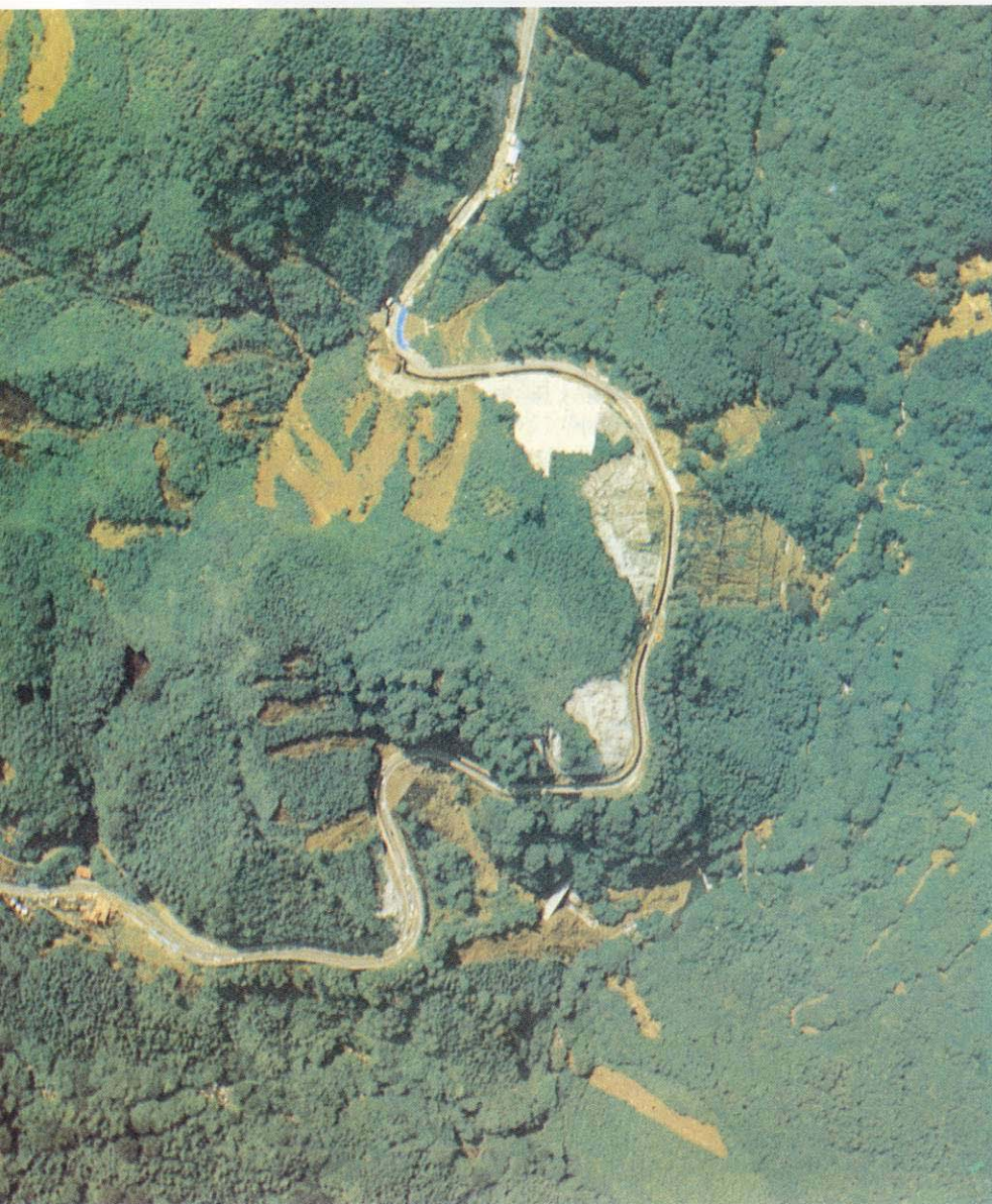
Surficial slides by heavy rainfalls after the earthquake in the same area as the photograph shown in the left page. (Air photograph taken on August 5, 1978)
