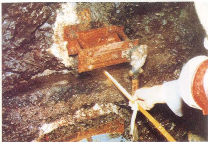
Slip surface and measurement of the displacement of the slide in the observation well (Washiodake landslide).
