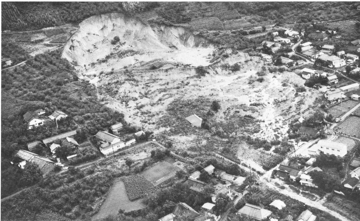
General view of Makiuchi landslide, caused by spring of much artesian water during earthquakes.
