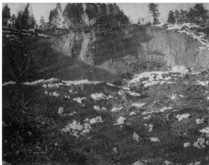
Main scarp at the top of landslide. Seepage water can be seen near the middle part of scarp. The sliding mass consists of mudstone.
