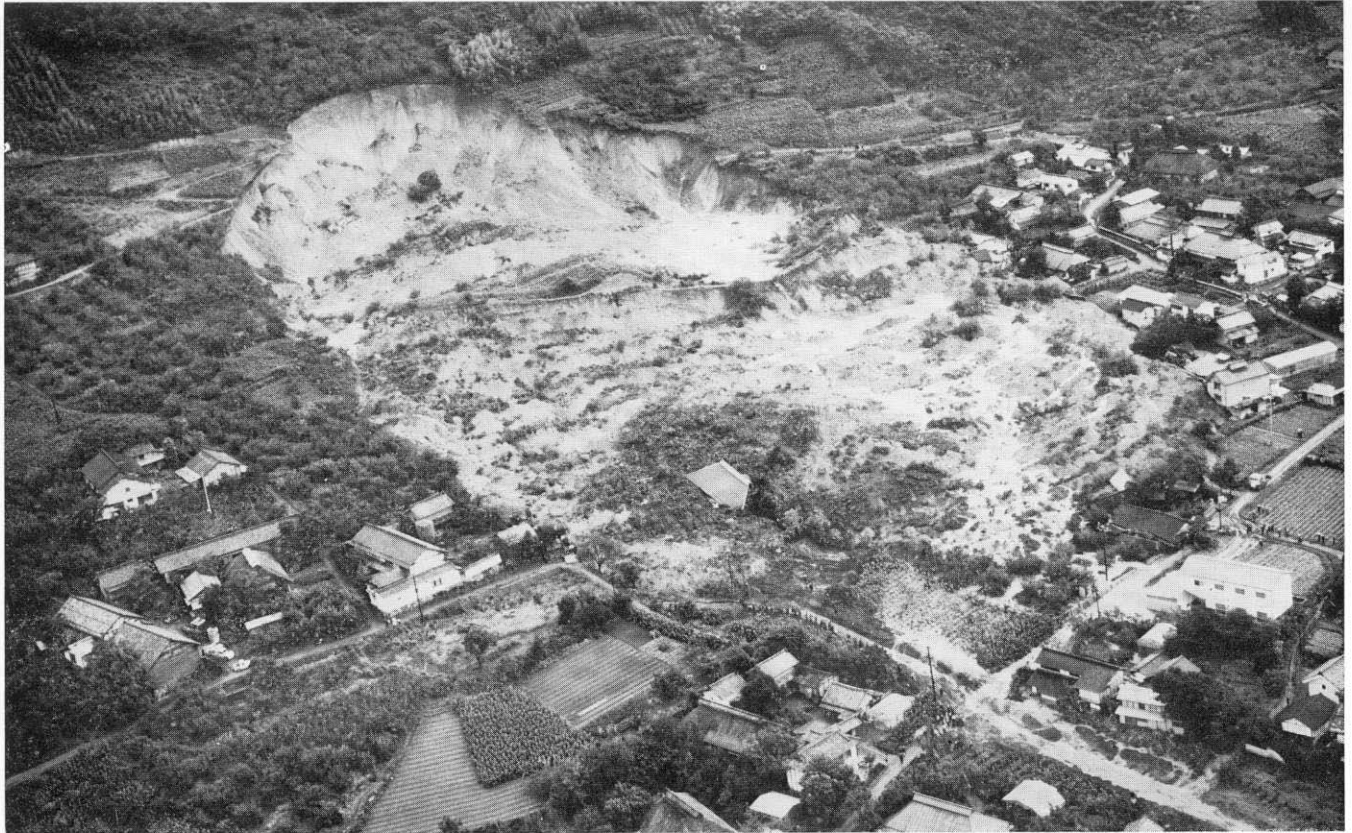
General view of slide caused by spring of much ground-water after earthquakes.
