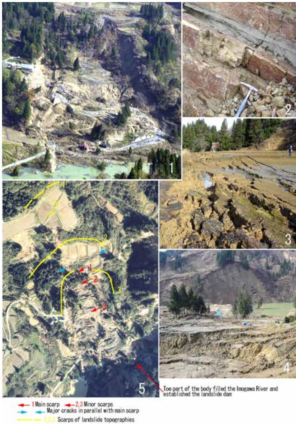
Fig.8 Geomorphic features of landslide at Terano site. 1. Overview of the landslide, 2. Close-up view of the bedrock, 3,4. Cracks cutting the ponds, 5. Interpretation of the aerial photograph of the landslide.
